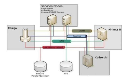
All the nodes are interconnected and with the BeeGFS cluster by an InfiniBand EDR high speed/low latency connection which provides a 100 Gb/s bandwidth. In addition to these there is also a 10 Gbit Ethernet network providing access to the users' home.
